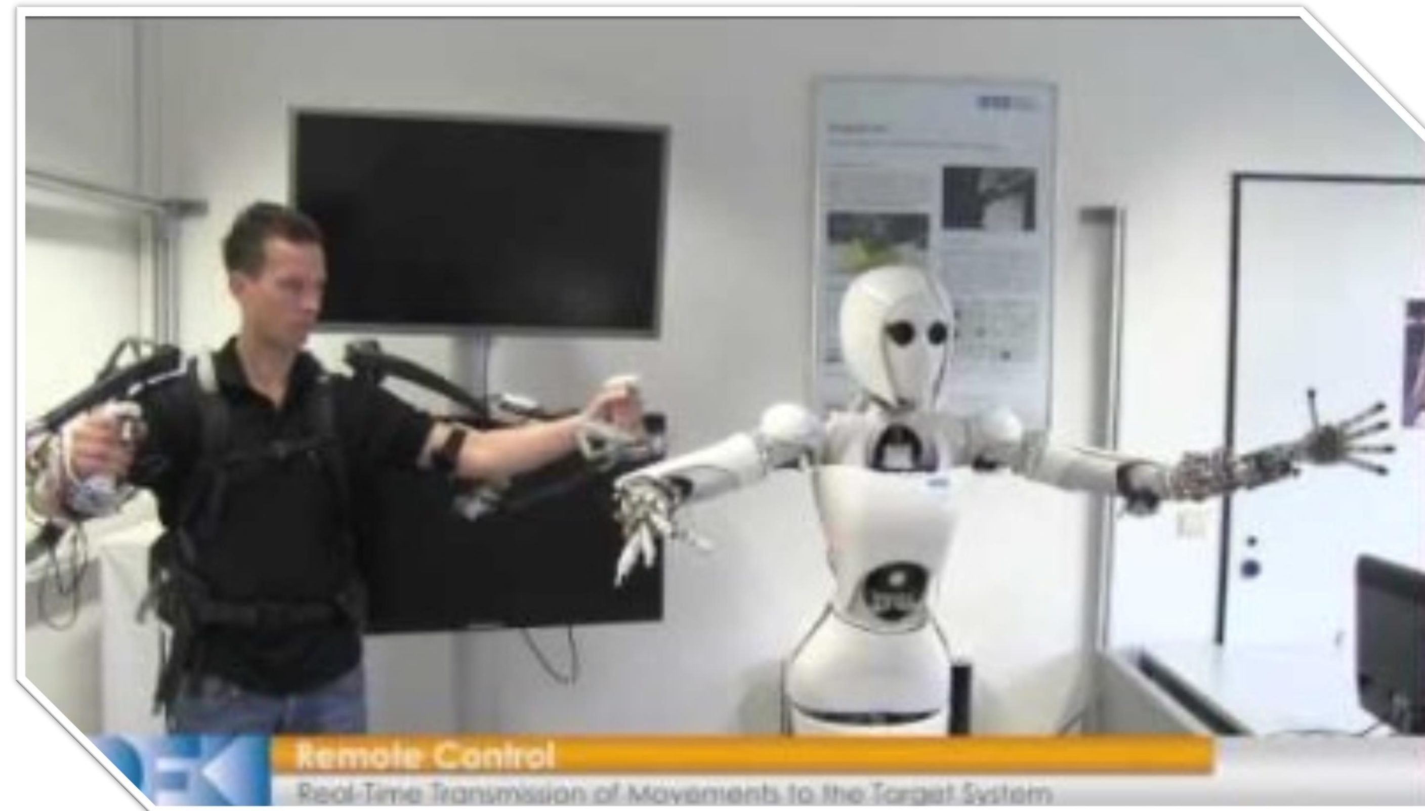
Capio Upper Body Exoskeleton for Teleoperation by the DFKI GmbH Robotics Innovation Center. https://robotik.dfki-bremen.de/en/research/projects/capio.html
