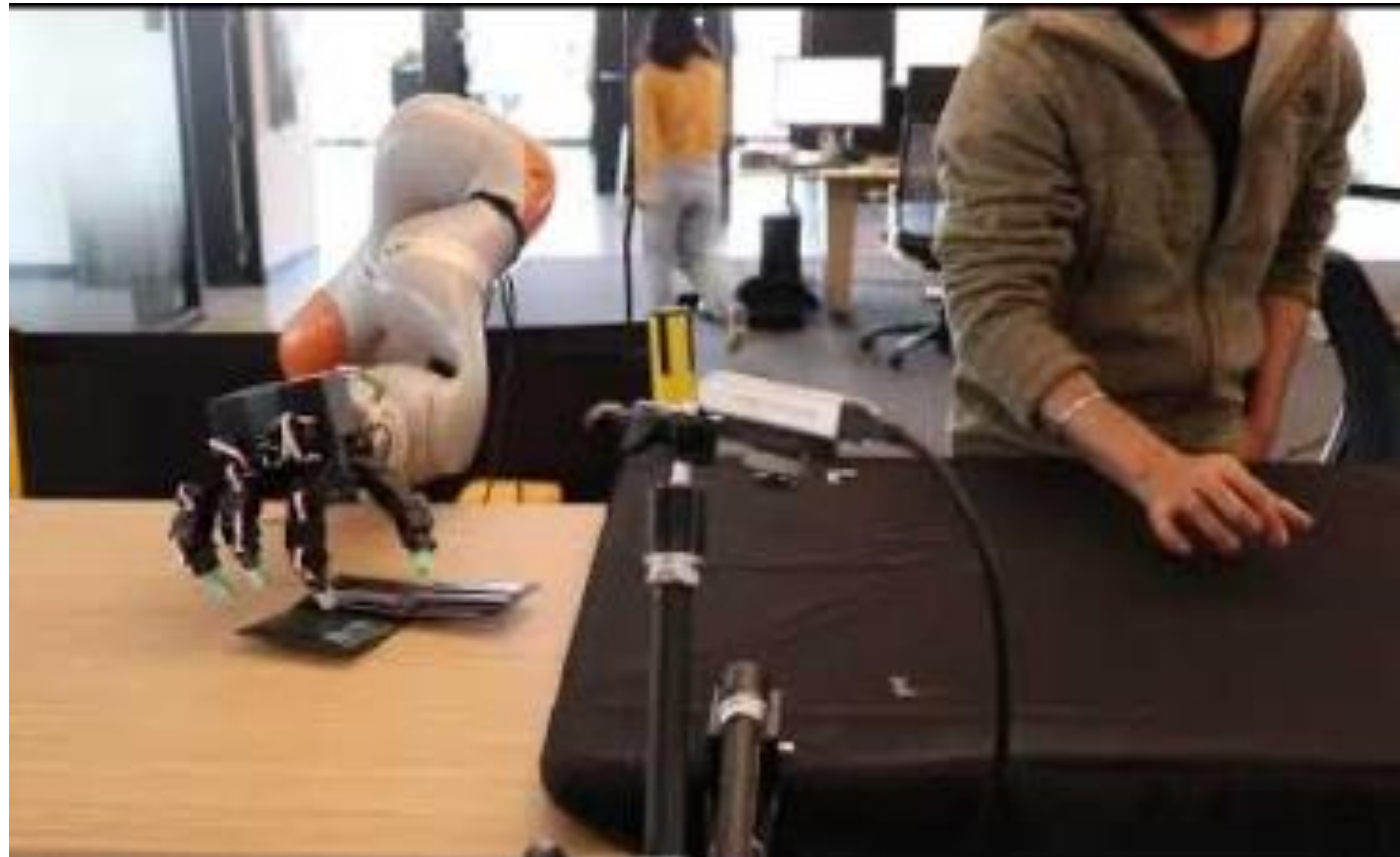
DexPilot: Vision Based Teleoperation of Dexterous Robotic Hand-Arm System Handa et al. ICRA 2020
