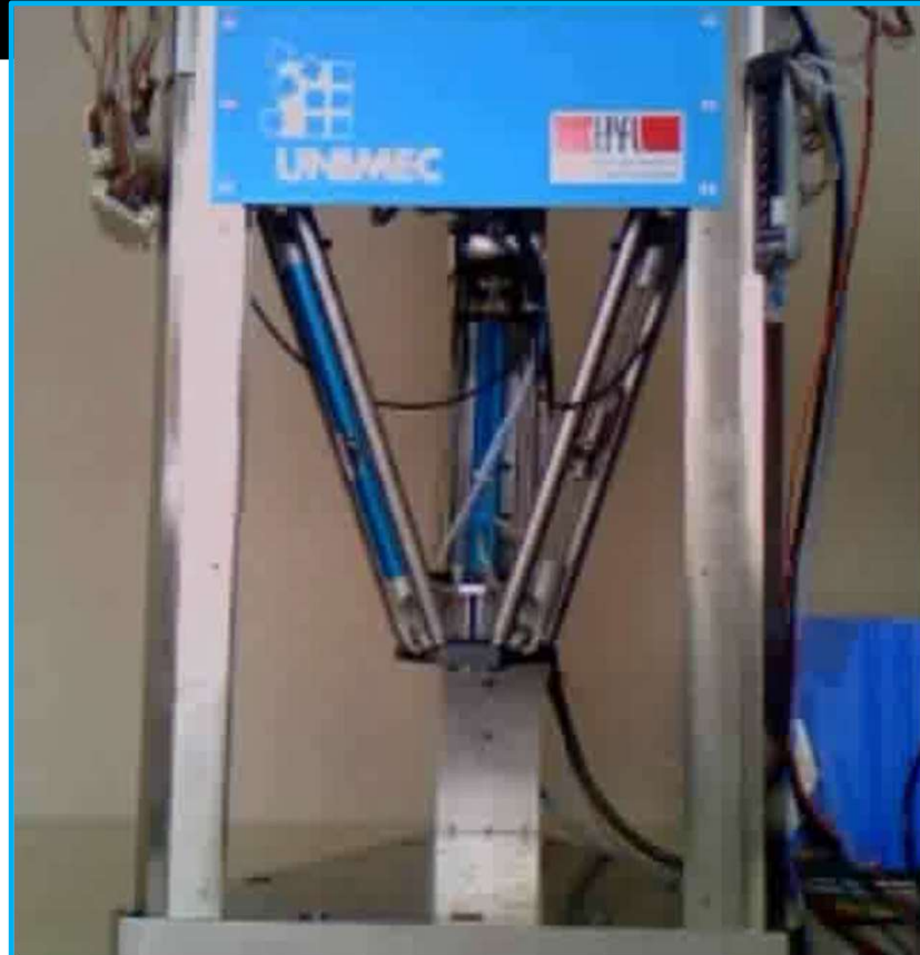
The Linear Delta - Vertical variant • Screw transmission
