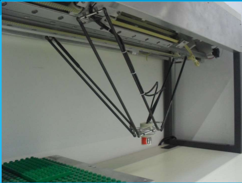
The Linear Delta - Horizontal variant • Belt transmission
