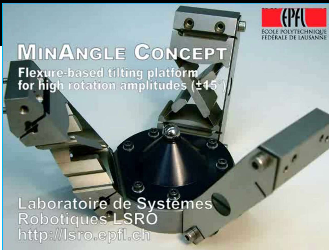
The Minangle – Ref. Flexible Hinges realization
