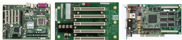
Figure 4.52, From Left to right, Industrial motherboard, passive PCI bus, PCI processor board (not motherboard)
