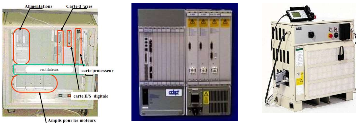
Figure 4.36, Examples of industrial numerical controller. From Left to right, EPFL robot controller, Adept controller and ABB controller
