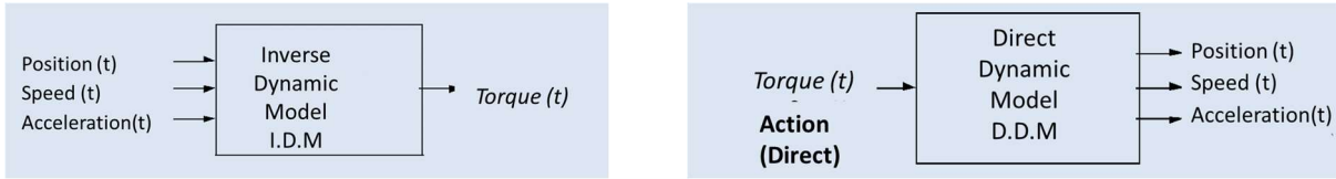
Figure 3.6. Forward and inverse dynamic models of a robot.
