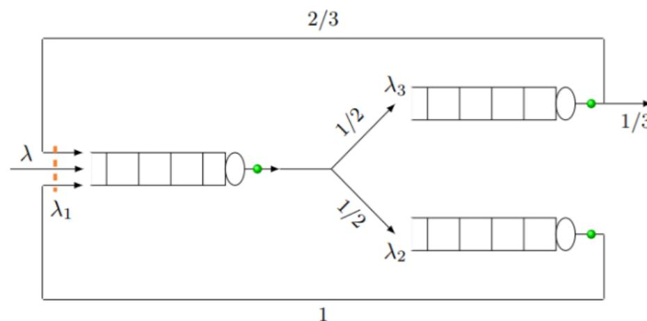
Figure 9.4: Open network with bifurcation and loop.
