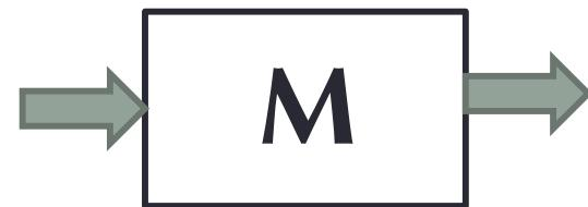
$0 \leq \text{Production rate } u \text{ of } M \leq \text{Capacity } U$
