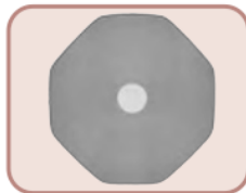
Structure of Octagonal ER Fibers
