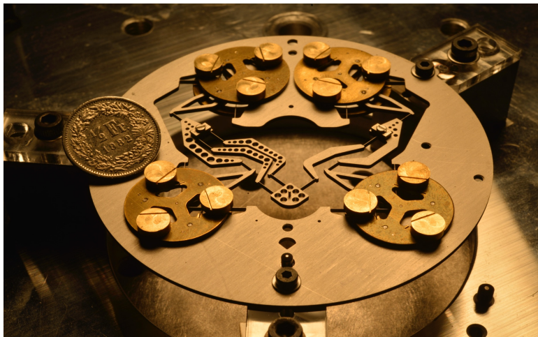
Wattwins titanium prototype (external diam. 75 mm)
