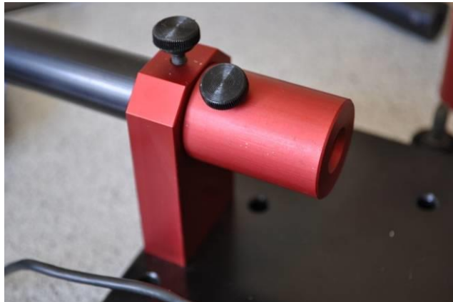
Figure 26. If the slit cap is put in contact with the source holder a good definition of the slit position is achieved. This is important because the sources will be exchanged!
