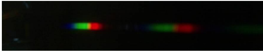
Figure 12: First and second diffraction orders for a white light source.
