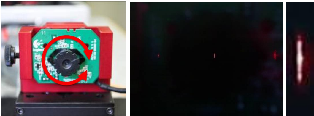
Figure 28. Same as Fig. 27 but with the slit in focus. On the very right the magnified image of the slit is given to show the focalisation.
