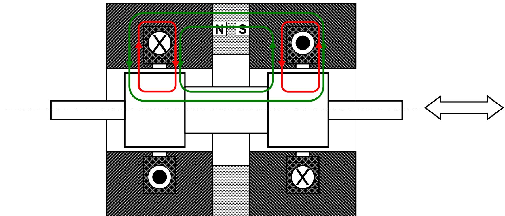
$$F_x = \frac{1}{2} \frac{dL_b}{dx} i_b^2 + \frac{1}{2} \frac{d\Lambda_a}{dx} \theta_a^2 + \frac{dL_{ab}}{dx} i_b \theta_a$$
