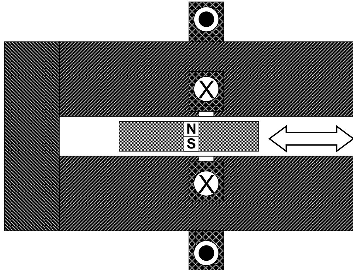
$$F_x = \frac{1}{2} \frac{d\Lambda_a}{dx} \theta_a^2 + \frac{dL_{ab}}{dx} i_b \theta_a$$
