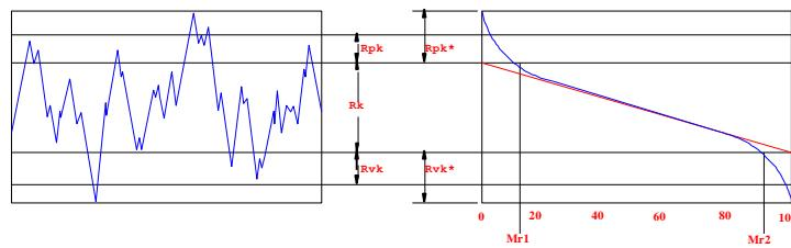
**Core Roughness, *Rk*,** is the core height of the profile along the Y-axis of the BAC curve generated by placing a 40% line on the curve at the minimum slope point and extending the lines to the 0% and 100% points.
