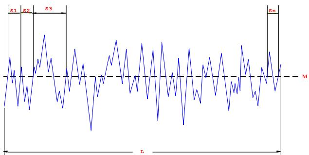
**Mean Spacing of Profile Irregularities, *Sm*,** is the mean value of the spacing between profile irregularities within the evaluation length.
