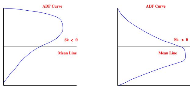
**Skewness, *Rsk*,** is a measure of the asymmetry of the profile about the mean line. A negative skewness indicates that a greater percentage of the profile is above the mean line and a positive value indicates that a greater percentage is below the mean line.
