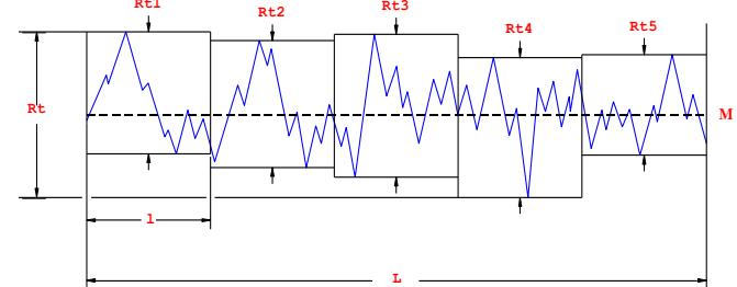
**Maximum Height of the Profile,  $Rt$** , the vertical distance between the highest and lowest points of the profile within the evaluation length.
