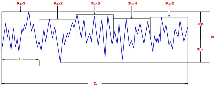
**Maximum Profile Peak Height,  $Rp$** , the distance between the highest point of the profile and the mean line within the evaluation length.
