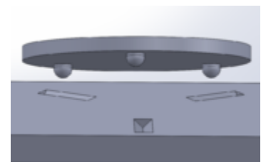
Figure 24. Schematic of a Maxwell coupling realized with a detachable cylindrical element.
