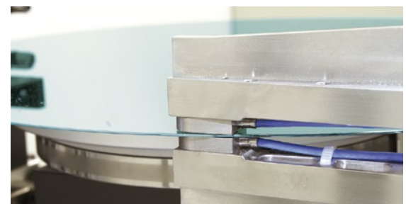
Wafer thickness measurement with two capacitive sensors
