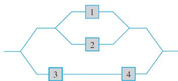
Let  $A_i$  denote the event that component # $i$  works ( $i = 1, 2, 3, 4$ ). Based on the design of the system, the event “the system works” is  $(A_1 \cup A_2) \cup (A_3 \cap A_4)$ . We’ll eventually need  $P(A_1 \cup A_2)$ , so work that out first:  $P(A_1 \cup A_2) = P(A_1) + P(A_2) - P(A_1 \cap A_2) = (.9) + (.9) - (.9)(.9) = .99$ . The third term uses independence of events. Also,  $P(A_3 \cap A_4) = (.8)(.8) = .64$ , again using independence.
