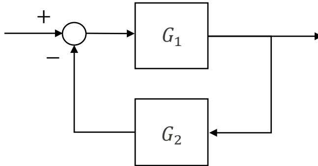
The **small gain theorem** ensures stability when the product of the  $\mathcal{L}_2$ -gains of two interconnected systems is less than one.
