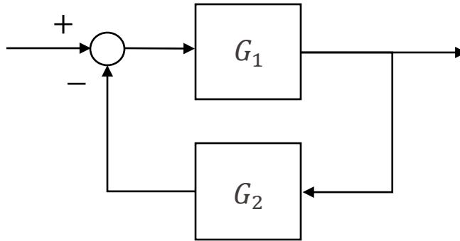
If both systems are strictly passive, the **passivity theorem** tells us that interconnection is passive and stable<sup>[\*]</sup>.
