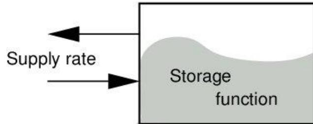
$$V(x(t_1)) \leq V(x(t_0)) + \int_{t_0}^{t_1} s(u(t), y(t)) dt.$$
