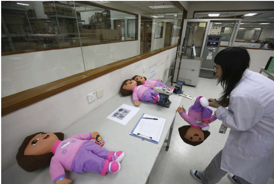
A Mattel technician in China does a pulling test with a Dora the Explorer doll in the name of product safety. Mattel has 10 labs in six countries and has set up strict requirements for vendors because of safety recalls.
