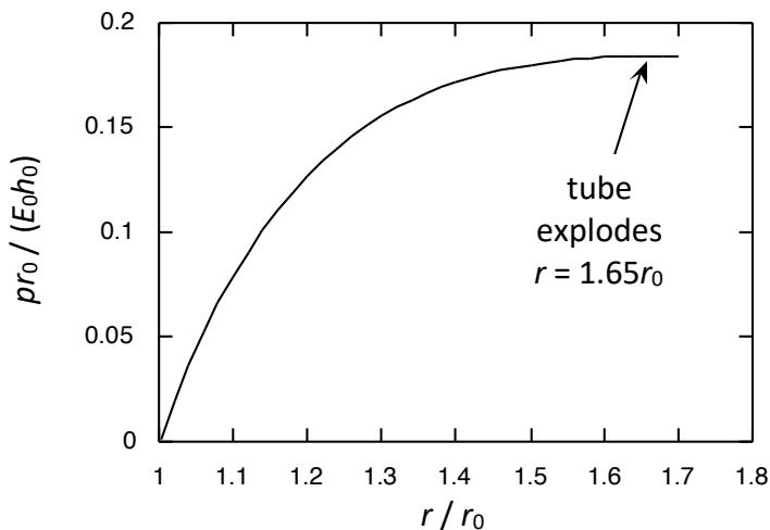
Note that at  $r/r_0 = 1.65$  the tube explodes (slope becomes zero).
