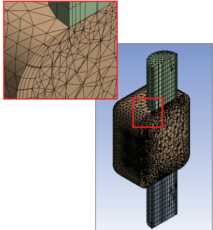
*Please Note: For continuous inflation without stair-stepping for this model, we have to unite all 3 bodies and use Multizone option. For MultiZone ref. slide No. 19*
