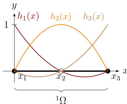
Inserting these expressions into the coefficients  $m_{ij}$  and  $k_{ij}$  of the mass and stiffness matrices leads, after integration, to the system of equations:
