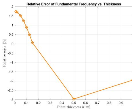
The discrepancy between the exact and approximate fundamental frequencies, especially for very thin or very thick plates, is due to the limitations of the plate theory and finite element modeling assumptions used in the analysis.
