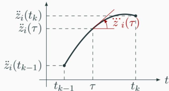
Notice that terms in  $\ddot{z}_i(\tau)$  and higher are neglected because they are multiplied in displacement by  $\Delta t^3$ , and in velocity by  $\Delta t^2$ .
