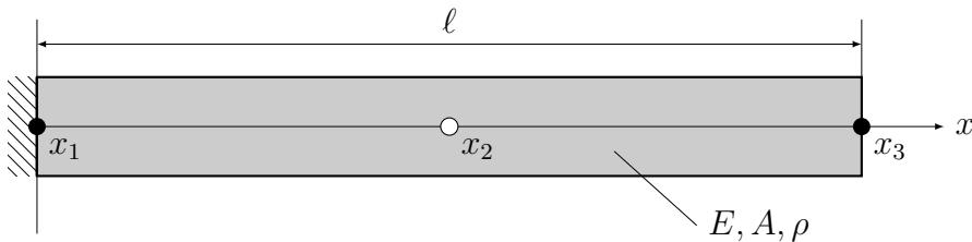
Assuming a diagonal lumped mass matrix obtained by summing the columns of the consistent mass matrix, the structure stiffness and lumped mass matrices are given by:
