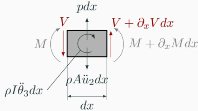
$$\begin{aligned}\partial_x \mathbf{V} + p &= \rho A \ddot{u}_2 \\ \partial_x M + \mathbf{V} &= \rho I \ddot{\theta}_3\end{aligned}$$
