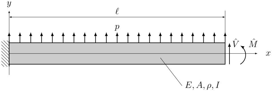
Given the strong form of the governing equations of motion, determine the weak form describing the transversal vibrations of the beam governed by the Timoshenko beam theory, which accounts for both shear deformation and rotary inertia.
