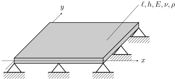
a) Model, using the finite element method, a square, isotropic, thin plate that is simply supported along all four edges using two  $n \times n$  meshes, one using AMC plate bending elements and the second using CR plate bending elements. The geometrical and material properties of the plate are given as:
