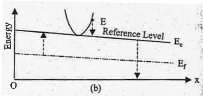
The Seebeck coefficient is a measure of the average heat current carried per electron.
