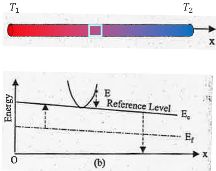
Let's now consider again our conductor subject to an electric field and a temperature gradient and let's look at the energy deposited in a differential volume due to the heat flux variation and the electrochemical potential drop:
