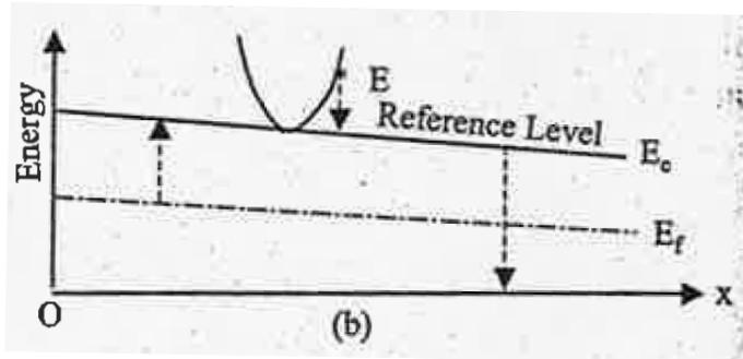
$$f = f_0 + \tau v_x \frac{\partial f_0}{\partial E} \left[ \frac{dE_f}{dx} + \frac{E - E_f}{T} \frac{dT}{dx} + e\mathcal{E} \right]$$
