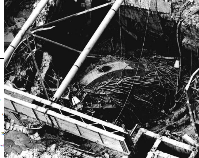
Upper reactor support plate with torn cooling channels
