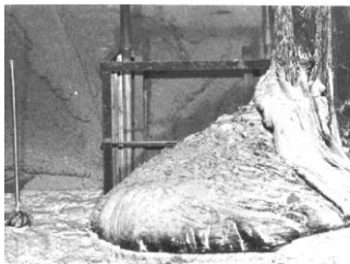
Refrozen corium melt "Elephant's foot"
