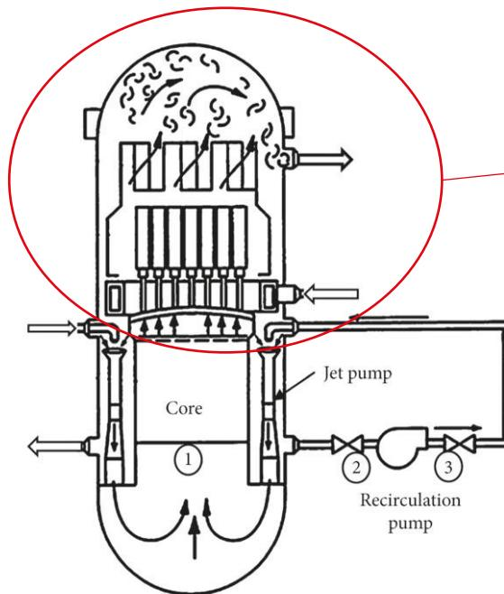
The steam is purified by water separators to obtain a very high steam quality in the turbine (>99.75%)
