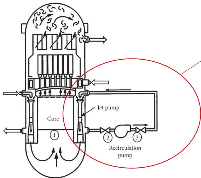
The non-evaporated water is **recirculated** by an external circuit and is re-injected in the vessel by **jet pumps** which create extra suction → this decreases the necessary pumping power
