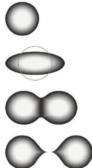
Stages of nuclear fission according to the Liquid Drop Model of the nucleus
