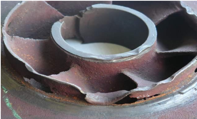
Figure 6: Cavitation erosion on turbine blades
