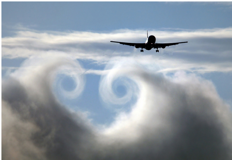
Figure 1. Two counter rotating vortices, induced by wing tips.
