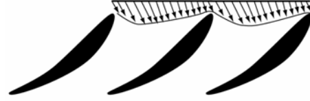
Flow field distortion due to guide vane wake
