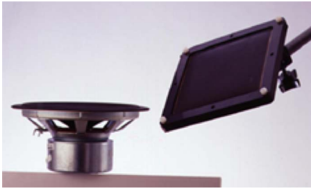
FIG. 11. (Color online) Flat foam-backed EAP loudspeaker (right) compared to a conventional electromagnetic moving-coil loudspeaker (left). The EAP loudspeaker is approximately 15 cm on a side (see Ref. 33).
