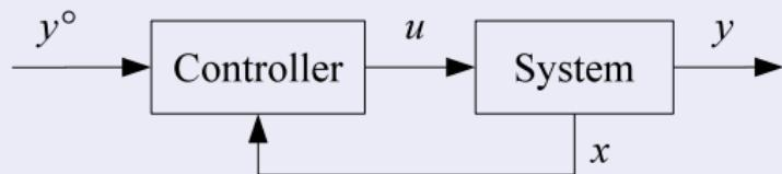
**State feedback**: the controller uses the setpoint and a measurement of the state for computing the control variable
