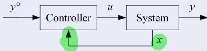
**State feedback:** the controller uses the setpoint and a measurement of the state for computing the control variable
