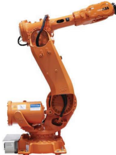
**Procedure** : The excitation signals are added to the joint torques and the joint angles  $q$ , joint speeds  $\dot{q}$  and joint accelerations  $\ddot{q}$  are measured. Then the parameters of the matrices  $M$ ,  $C$  and  $G$  can be identified with the least squares algorithm.
