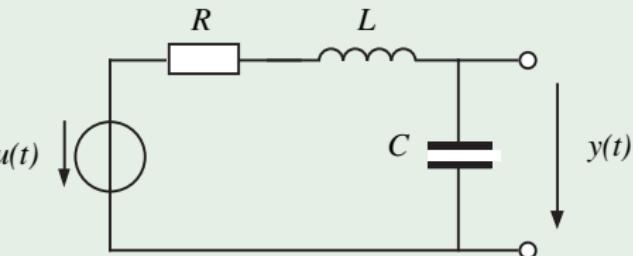
$$\begin{aligned} x_1(t) &\equiv i_L(t) \Rightarrow R x_1(t) + L \dot{x}_1(t) + x_2(t) = u(t) \\ x_2(t) &\equiv u_C(t) \Rightarrow x_1(t) = C \dot{x}_2(t) \end{aligned}$$
