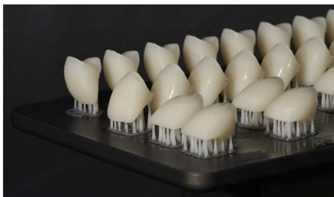
Figure 5.2: Temporary crowns fabricated using Digital Light Processing (DLP) technology
