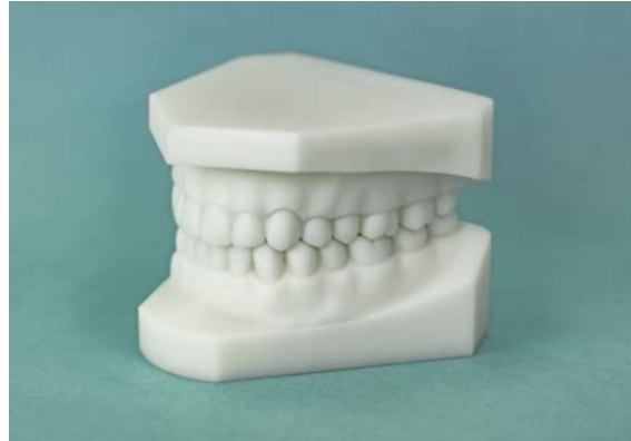
Figure 2.1: Example of a dental model made by 3D resin printing [3]
