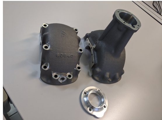
Figure 6: New Ferrari 340 Barchetta's rear transmission made by SLM
