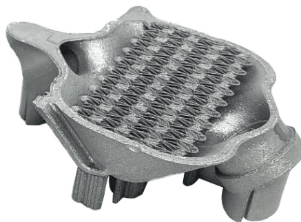
Figure 17: Velo3D printed heat exchangers featuring 320 \mu\text{m} leak-tight walls and 220 \mu\text{m} turbulators that resulted in lower pressure drop [6]
