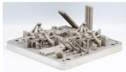
Figure 11: Plate after SLM process
