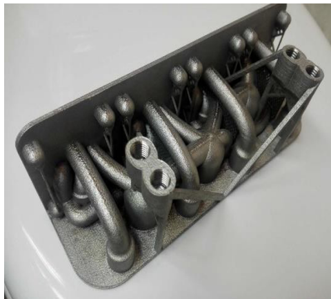
Figure 19: 3D printed metal hydraulic manifolds, optimizing weight and volume [7]
