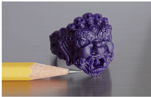
Figure 8: Detailed part made with SLA[16].
