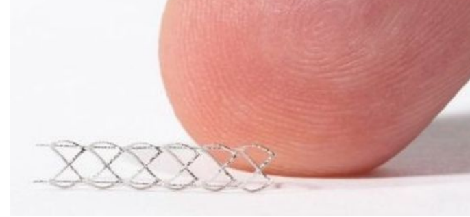
Stents manufactured with \mu SLM[3]
