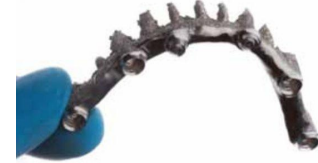
Ti mandibular framework fabricated using EBM technology [1]
