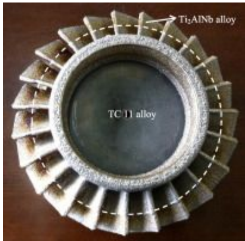
Direct laser deposited TC11/Ti 2 AlNb dual alloy blisk for aero engines
