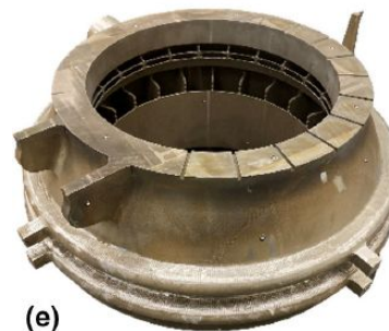
L-PBF Inconel 718 integrated heat exchanger
