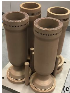
L-PBF GRCo-84 combustion chambers
