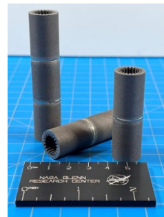
L-PBF C-103 heat pipe segments
