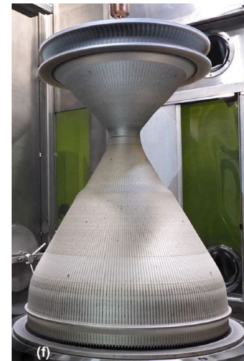
LP-DED Nasa HR-1 Nuclear thermal propulsion chamber
