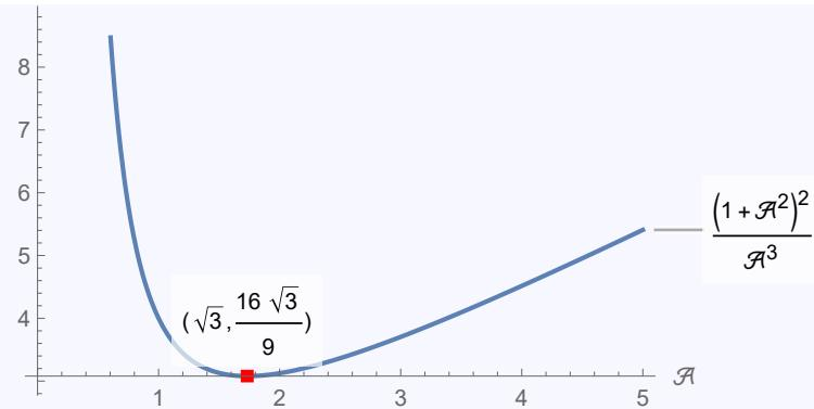
Hence, the critical shear is minimized at an aspect ratio of  $a = \sqrt{3}b$ , with value
