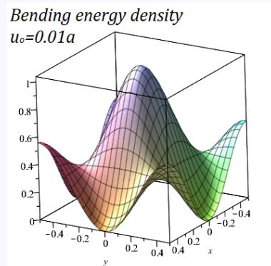
4. Using the curvature components  $\mathcal{K}_{\alpha\beta}$  computed in question 2, calculate the total bending energy (assuming  $D$  is the bending stiffness of the plate). Your answer should be proportional to  $\tilde{w}^2/a^2$ .
