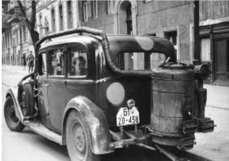
A German car with gasification (1946)
