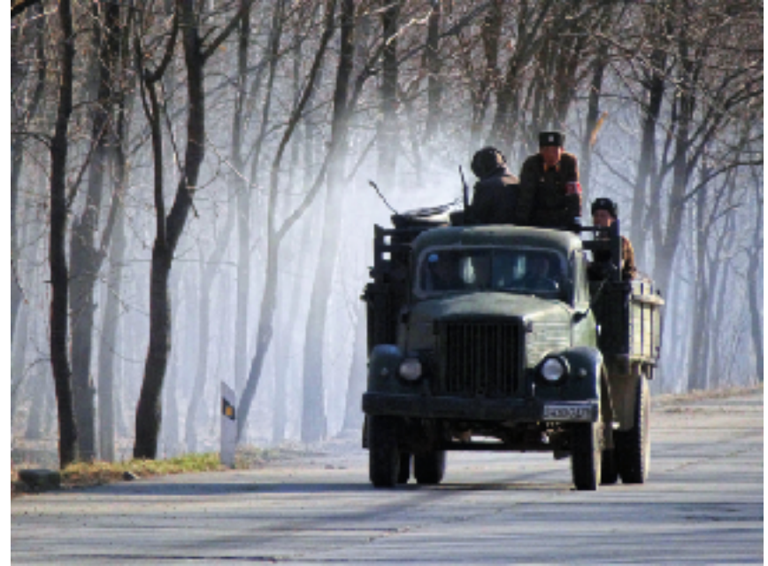
A North-Korean truck with gasification (2014)
