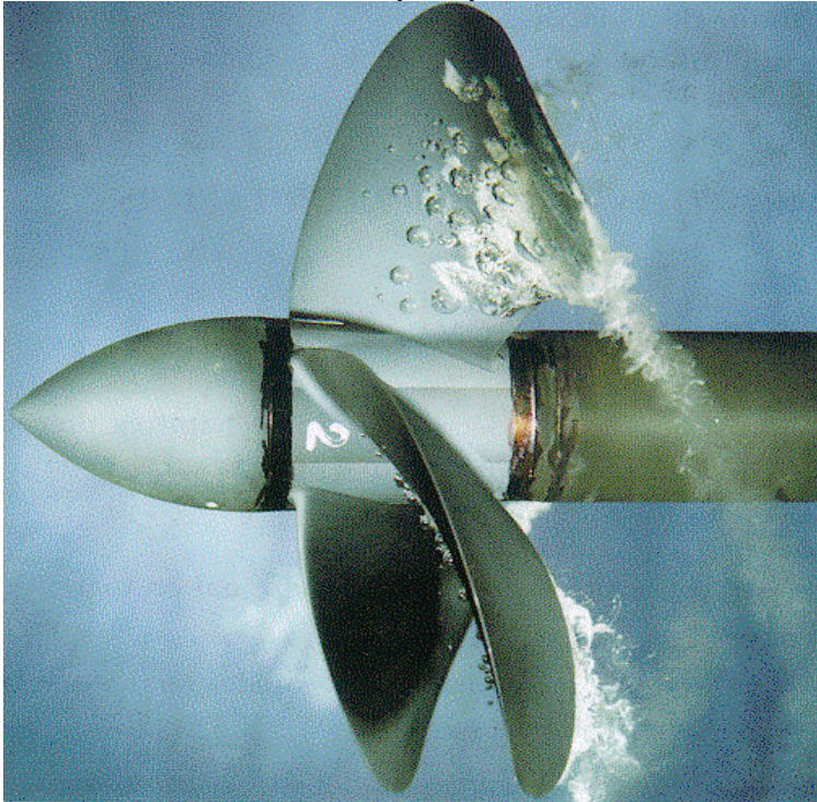
Bubble Cavitation in a marine propeller
