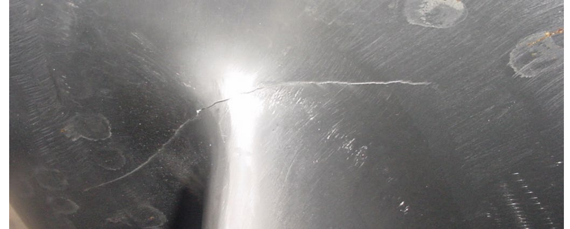
Premature cracks in a 200 MW Pump Turbine
