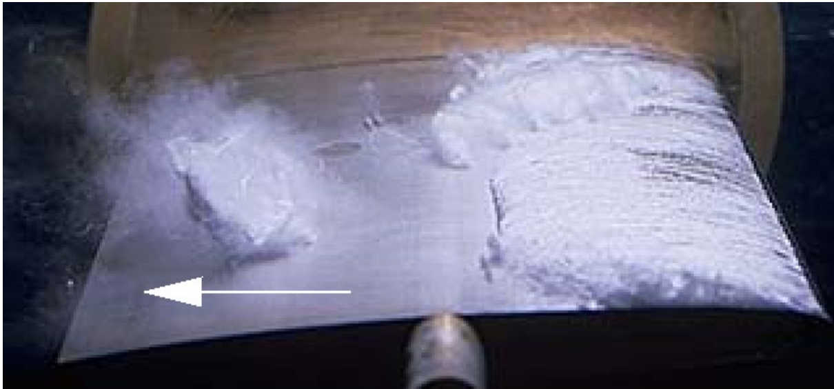
Side view of attached cavitation on a 2-D hydrofoil
