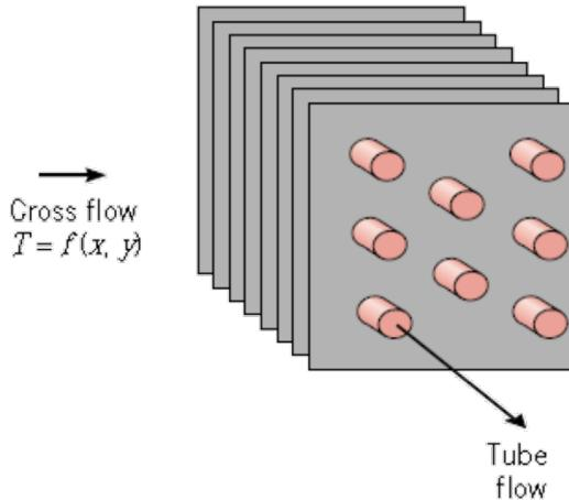
$$\frac{1}{U A} = R_{conv,out} + R_{foul,out} + R_{cond} + R_{foul,in} + R_{conv,in}$$
