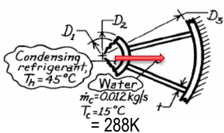
$$\begin{aligned} D_1 &= 10\text{ mm} \\ D_2 &= 14\text{ mm} \\ D_3 &= 50\text{ mm} \\ t &= 2\text{ mm} \end{aligned}$$
