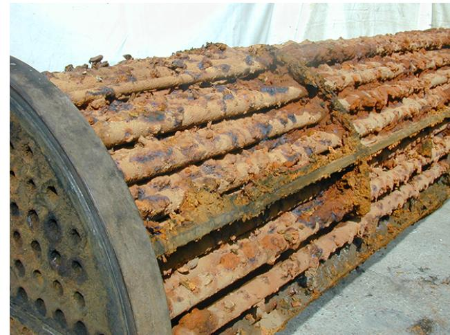
Dramatic increase in thermal resistance due to poor conduction through the scaling layer
