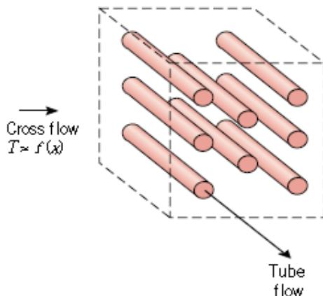
$$\frac{1}{U A} = R_{conv,out} + R_{foul,out} + R_{cond} + R_{foul,in} + R_{conv,in}$$
