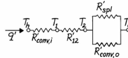
To estimate the thermal resistance on the water side (c), first evaluate the convection coefficient. The hydraulic diameter for a passage, where  $A_c$  is the cross-sectional area of the passage is
