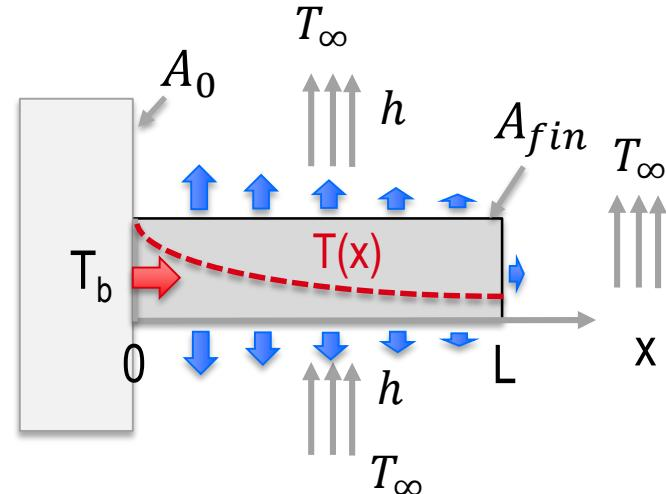
e.g. for infinite fin we get:  $R_f \equiv \frac{\theta_b}{Q_f} = \frac{\theta_b}{M} = \frac{1}{\sqrt{hPkA_c}}$
