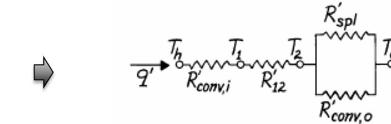
To estimate the thermal resistance on the water side (c), first evaluate the convection coefficient. The hydraulic diameter for a passage, where  $A_c$  is the cross-sectional area of the passage is
