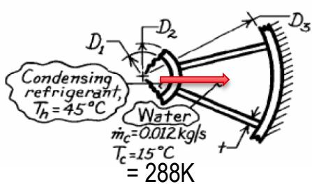
$$\begin{aligned} D_1 &= 10\text{ mm} \\ D_2 &= 14\text{ mm} \\ D_3 &= 50\text{ mm} \\ t &= 2\text{ mm} \end{aligned}$$
