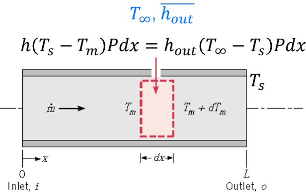
Often the surface temperature is maintained constant with forced external convection, hence using a fluid with known  $T_{\infty}$
