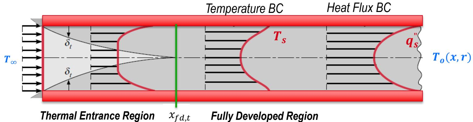
$$\left. \frac{\partial \theta}{\partial x} \right|_{x=x_{fd,t}} \equiv 0 \quad \rightarrow \quad \left. \frac{\partial T}{\partial x} \right|_{x=x_{fd,t}} = \left. \frac{dT_s}{dx} \right|_{x=x_{fd,t}} - \left. \frac{T_s - T}{T_s - T_m} \frac{dT_s}{dx} \right|_{x=x_{fd,t}} + \left. \frac{T_s - T}{T_s - T_m} \frac{dT_m}{dx} \right|_{x=x_{fd,t}}$$
