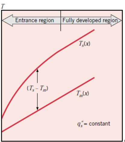
For a constant heat flux  $q_s''$  we have:  $\frac{dT_m}{dx} = \frac{q_s'' P}{\dot{m} c_p} \rightarrow T_m(x) = \frac{q_s'' P}{\dot{m} c_p} x + T_{m,i}$
