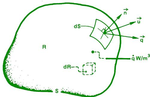
$$\dot{U} = \dot{m} \left( u + pv + \frac{1}{2}V^2 + gz \right)_{in} - \dot{m} \left( u + pv + \frac{1}{2}V^2 + gz \right)_{out} + \dot{Q} - \dot{W} + \dot{E}_{gen}$$
