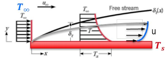
$$Nu_{\textcolor{red}{L}} = \frac{hL_c}{k_f} = \frac{\partial \left( \frac{T_s - T}{T_s - T_\infty} \right)}{\partial \left( \frac{y}{L_c} \right)} \Bigg|_{y/L_c=0}$$
