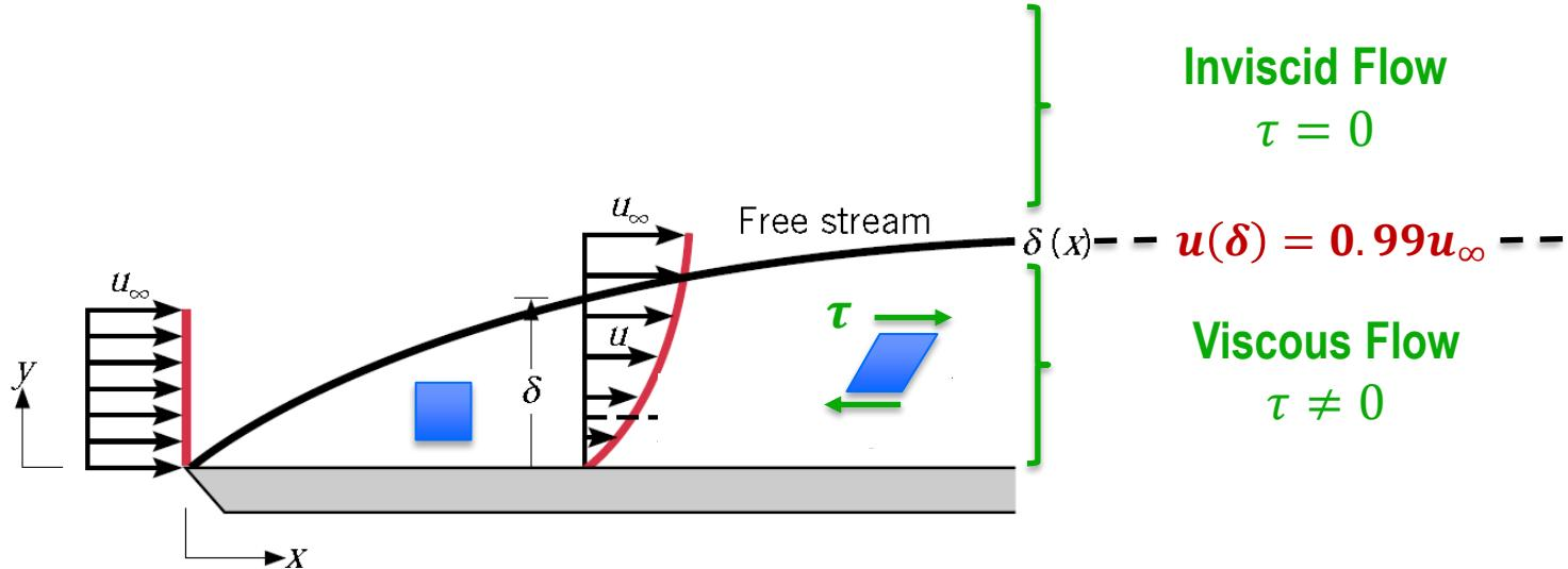
**Shear stress  $\tau$  = friction force per unit area**
