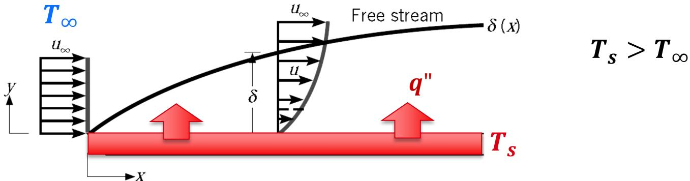
**Newton's law:** the heat transfer is proportional to the temperature difference between the wall and the unperturbed fluid
