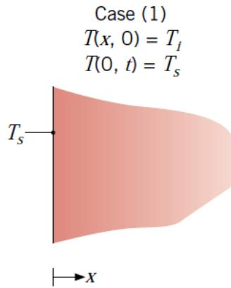
$$\frac{T - T_s}{T_i - T_s} = (2/\pi^{1/2}) \int_0^\eta \exp(-u^2) du \equiv \text{erf } \eta$$
