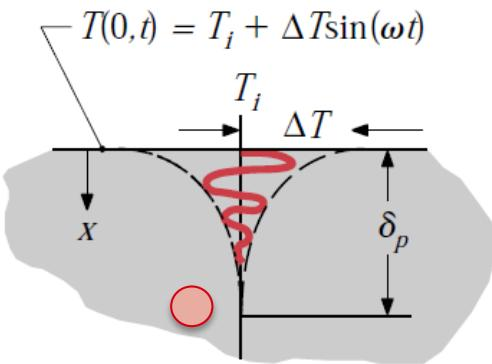
There are many situations in which the surface temperature or the heat flux change periodically (e.g. seasonal temperature variation of soil temperature, periodic heat dissipation in electronic chips)
