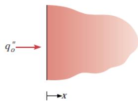
$$T(x, t) - T_i = \frac{2q_o''(\alpha t / \pi)^{1/2}}{k} \exp\left(\frac{-x^2}{4\alpha t}\right) - \frac{q_o'' x}{k} \operatorname{erfc}\left(\frac{x}{2\sqrt{\alpha t}}\right)$$
