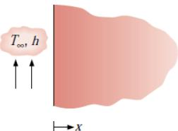
$$\frac{T(x, t) - T_i}{T_\infty - T_i} = \operatorname{erfc}\left(\frac{x}{2\sqrt{\alpha t}}\right) - \left[ \exp\left(\frac{hx}{k} + \frac{h^2 \alpha t}{k^2}\right) \right] \left[ \operatorname{erfc}\left(\frac{x}{2\sqrt{\alpha t}} + \frac{h\sqrt{\alpha t}}{k}\right) \right]$$
