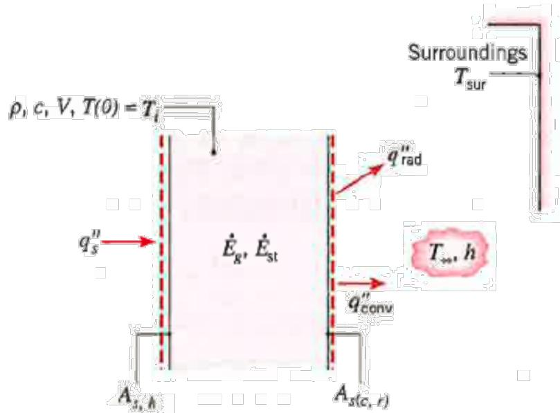
$$q''_s A_{s,h} + \dot{E}_g - [h(T - T_\infty) + \varepsilon\sigma(T^4 - T_{sur}^4)] A_{s(c, r)} = \rho V c \frac{dT}{dt} \quad (5.15)$$
