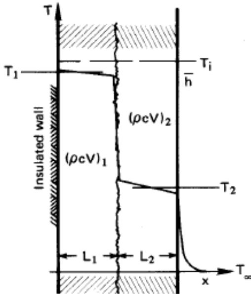
$$\text{slab 1 : } -(\rho cV)_1 \frac{dT_1}{dt} = \bar{h}A(T_1 - T_2)$$
