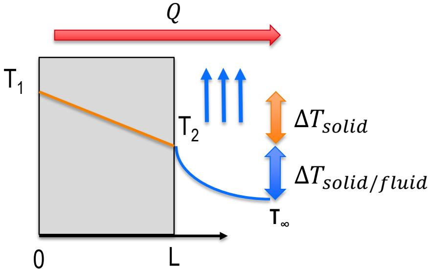
$$Q = \frac{(T_1 - T_2)}{R_{th,cond}} = \frac{(T_2 - T_\infty)}{R_{th,conv}}$$
