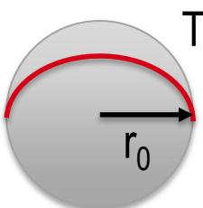
We defined the critical dimension  $L_c$  as the ratio of volume (heat capacity) and surface area (convection). However, with Bi we want to estimate how uniform the T profile is, so it is also reasonable to use as critical length the length over which the temperature profile might change (so for a sphere it would be  $r_0$ ).
