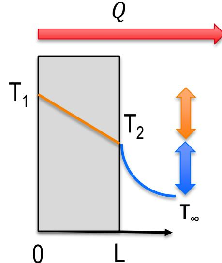
$$\Delta T_{solid} \sim \Delta T_{solid/fluid}$$
