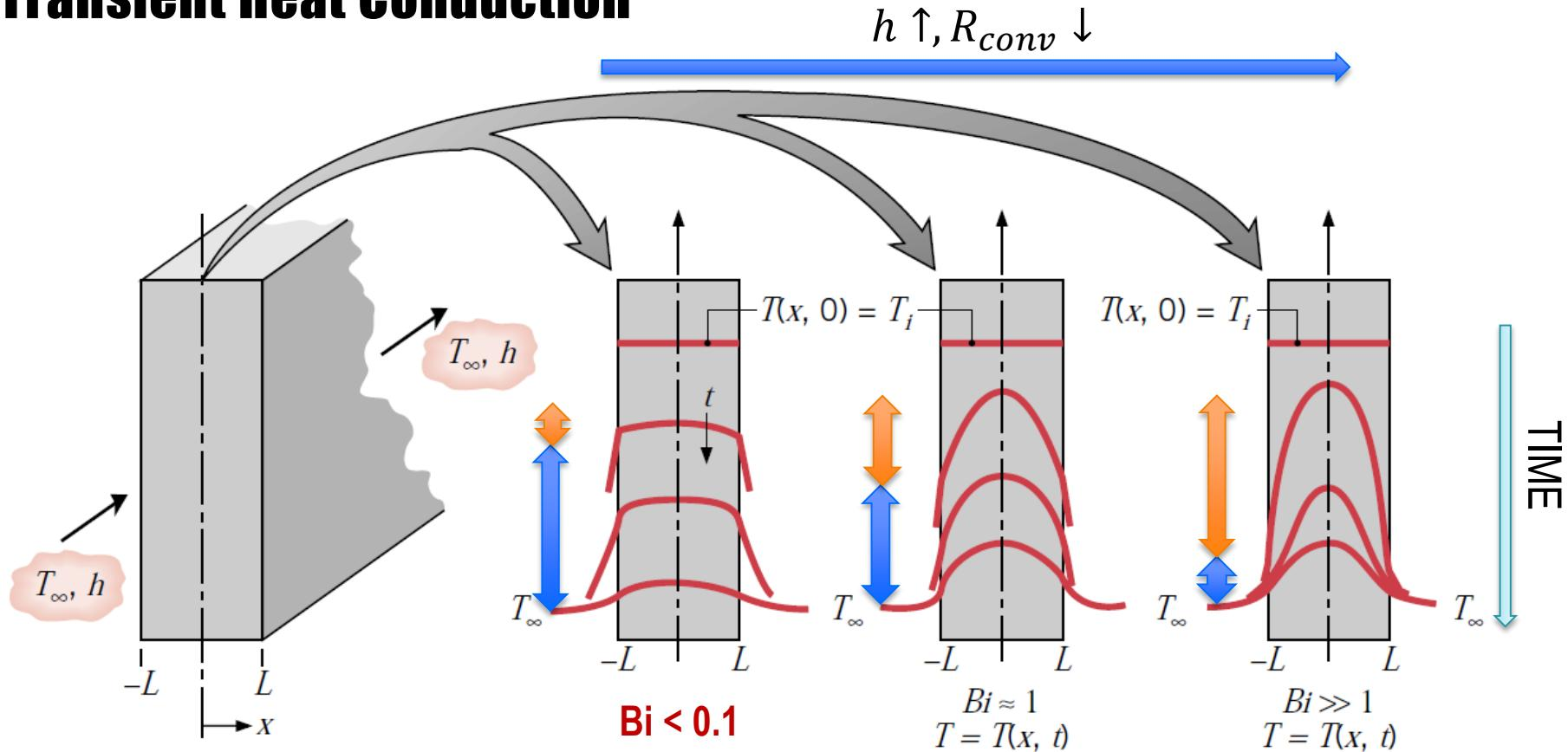
Note: during the transient the temperature is *NOT* linear within the wall even if there are no heat sources
