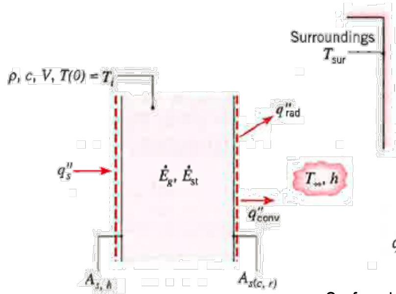
Can you find the transient solution if only radiative heat transfer is present, without heat sources?
