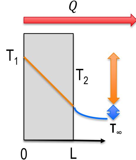
$$\Delta T_{solid} \gg \Delta T_{solid/fluid}$$
