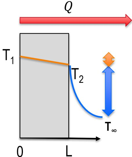
$$\Delta T_{solid} \ll \Delta T_{solid/fluid}$$
