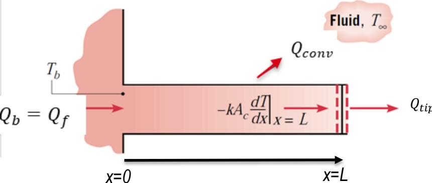
$$\frac{d^2\theta}{dx^2} - m^2\theta = 0 \quad \rightarrow \quad \theta = C_1 e^{mx} + C_2 e^{-mx}$$
