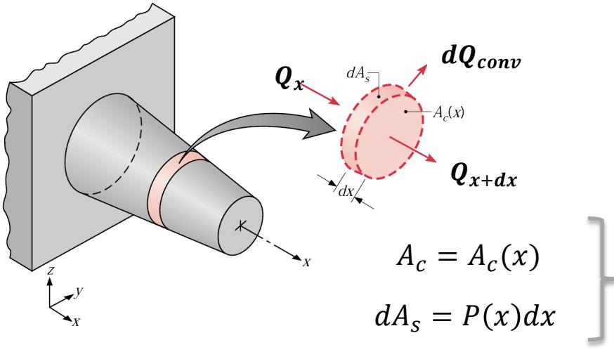
$$\left. \begin{aligned} A_c &= A_c(x) \\ dA_s &= P(x)dx \end{aligned} \right\}$$
