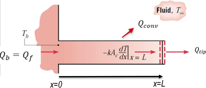
The fin was added to enable better heat transfer. So we want to know how much heat is being removed by the fin. We observe that convection on the fin can remove only as much heat as it initially enters the fin by conduction.
