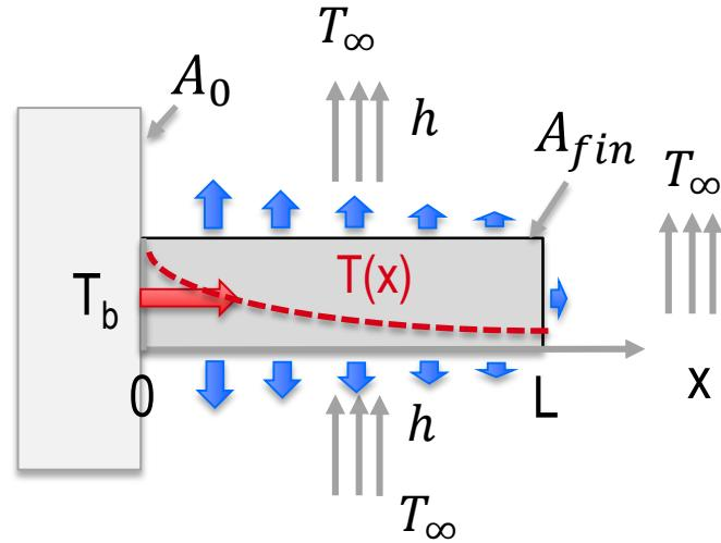
$$\eta_f \equiv \frac{Q_f}{Q_{f,max}} = \frac{Q_f}{hA_f(T_b - T_\infty)}$$
