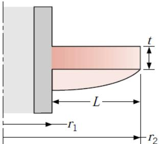
$$\eta_f = C_2 \frac{K_1(mr_1)I_1(mr_{2c}) - I_1(mr_1)K_1(mr_{2c})}{I_0(mr_1)K_1(mr_{2c}) + K_0(mr_1)I_1(mr_{2c})} \quad (3.91)$$
