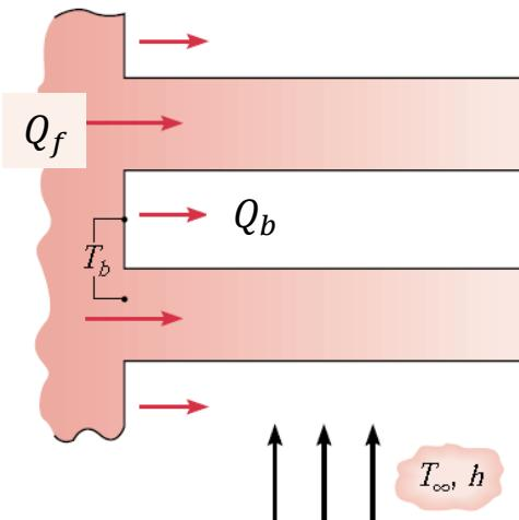
$$\eta_t \equiv \frac{Q_t}{Q_{t,max}} = \frac{Q_t}{hA_t(T_b - T_\infty)} = \frac{NQ_f + Q_b}{h(NA_f + A_b)(T_b - T_\infty)}$$
